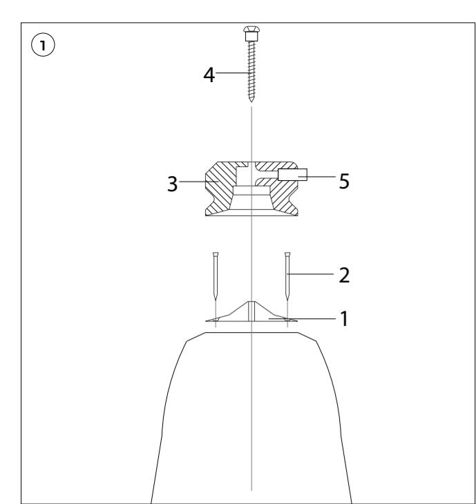
3. Screw the Bottom Attachment to the Guide with the Screw. Make sure that the exit hole, with the Dummy for the Lanyard Cord, is correctly positioned to ensure that the Lanyard operates with minimum friction.
